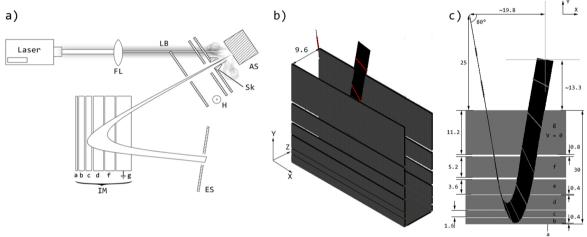
Fig. 1 (a) Ion optics scheme of laser ion source providing time focus. LB – laser beam, AS – sample, Sk – skimmer, IM – ion mirror, FL – focusing lens, ES – exiting slit, H – magnetic field vector. (b) Gridless ion mirror design. Isometric projection. (c) Gridless ion mirror design. XY projection. Letters a – g represent plate pairs.
