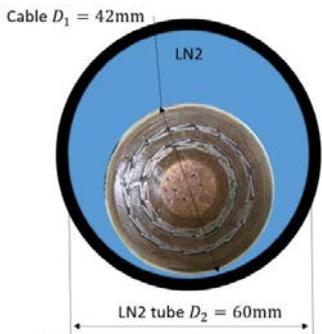
Fig. 1. Cross section of the inner part of the cable. The diameter of the cable is 42 mm, the diameter of the area with liquid nitrogen is 60 mm.
