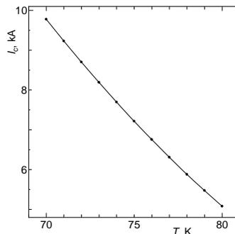
Fig. 2. The dependence of critical current of the cable made of 35 tapes of Bi2223. This dependence was recalculated from the experimental data from [5].
