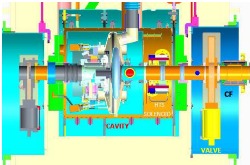
Fig. 1. SC RF electron gun cavity assembled in the gun cryostat. The HOM measured results depend on the status of the vacuum gate. For operation, the CF damper is replaced by a NC solenoid.
