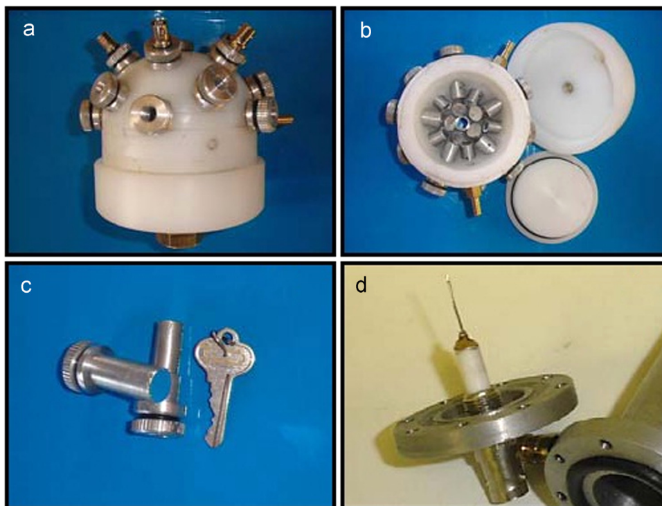
Fig. 1. (a) General view of detector, (b) open detector with sample holder, (c) NAPCs and (d) needles anode.
