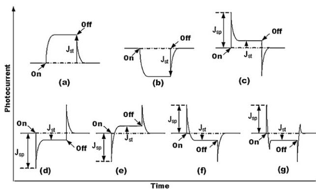
Fig. 2. Various patterns of transient photocurrent response for oxidation films formed on metal surface.
