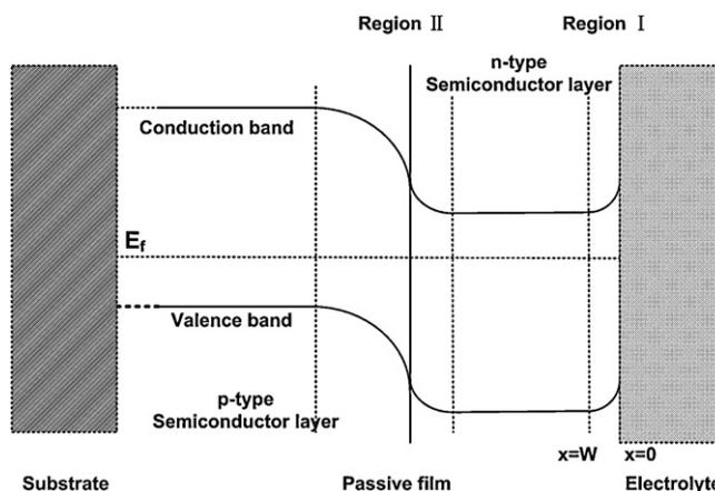
Fig. 1. Schematic illustration showing electronic structure of duplex oxide films formed on 304L SS in high temperature water.
