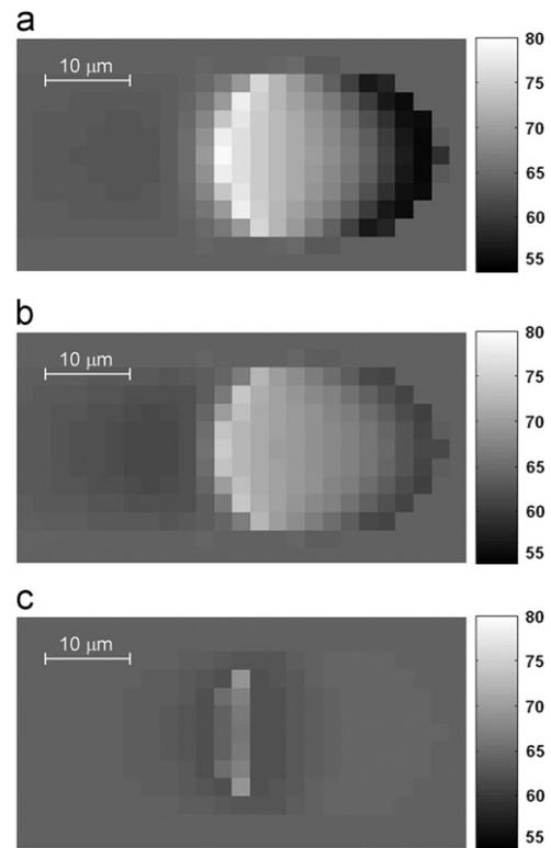
**Fig. 3.** Iron concentrations [%] in invar sample determined by 3 methods of quantitative analysis for geometry  $45^\circ/90^\circ$ . (a) Method based on direct comparison between count rate and concentration; (b) fundamental parameter method; (c) improved method using parameter  $\theta$ .
