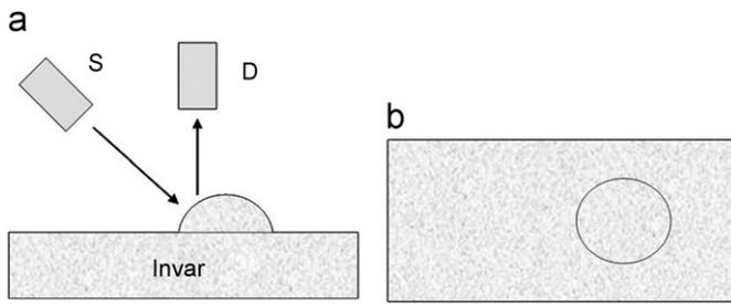
**Fig. 1.** (a) Simulation of 2D scanning of an invar alloy; the surface roughness is represented by a hemisphere 10  $\mu\text{m}$  in radius; S—X-ray source, D—detector (b) top view.
