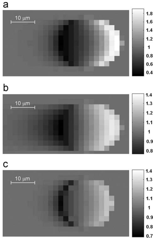
**Fig. 2.** Relative fluences of characteristic radiation determined with a Monte Carlo simulation of  $\mu$ -XRF scanning of invar sample. The position of an invar hemisphere on the smooth surface is indicated. (a)  $K\alpha$  line of nickel (geometry  $45^\circ/90^\circ$ ); (b)  $K\alpha$  line of iron (geometry  $45^\circ/90^\circ$ ); (c)  $K\alpha$  line of iron (geometry  $75^\circ/90^\circ$ ).
