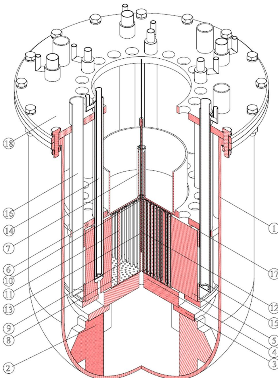
**Fig. 1.** MNSR isometric view; 1—reactor vessel, 2—reactor base, 3—lower orifice, 4—lower reflector, 5—annular reflector, 6—upper orifice, 7—upper shim tray, 8—lower grid plate, 9—fuel elements, 10—upper grid plate, 11—tie rod, 12—control rod, 13—control rod clad, 14—inner irradiation sites, 15—outer irradiation sites, 16—reactivity regulator, 17—core cover, 18—vessel cover.
