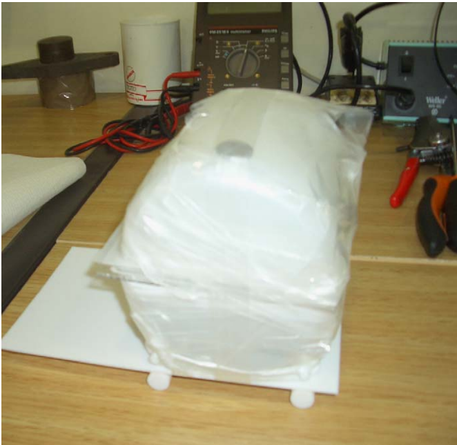
Fig. 2. Phantom utilised for the irradiation of gel dosimeter layers.
