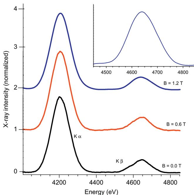
Fig. 2. A typical K X-ray spectrum of the Co target in  $B = 0$ ,  $B = 0.6$  T and  $B = 1.2$  T magnetic field. The spectra were plotted after smoothing.
