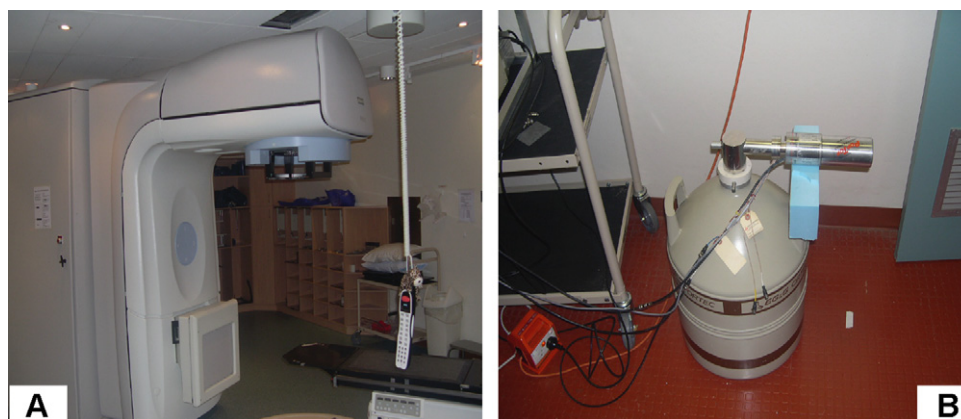
Fig. 1. Photograph (A) shows a medical linac similar to the one used in the experiments. Photograph (B) shows the HPGe detector, which is cooled by liquid nitrogen in a Dewar.
