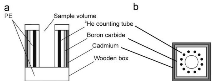
Fig. 1. Vertical (a) and horizontal (b) cross section view of the neutron detector arrangement used for DNAA at the TRIGA-Mainz facility.
