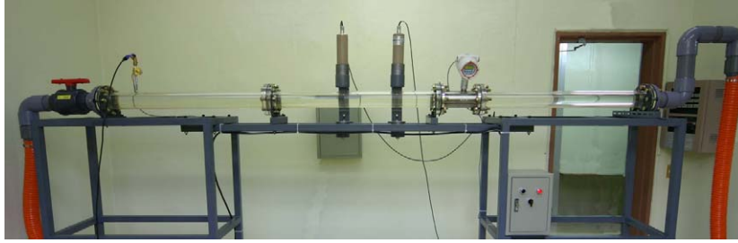
Fig. 1. Experimental set-up for sealed gamma radioisotope application to the measurements of velocity in a multi-phase flow.
