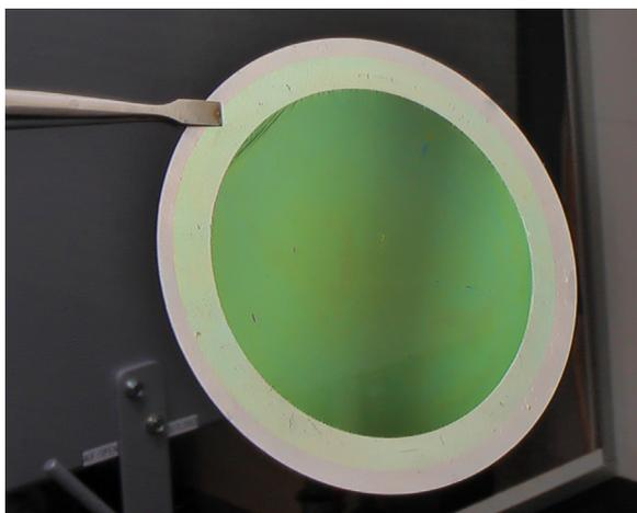
Fig. 1. Polyimide foil with an areal density of  $32 \mu\text{g cm}^{-2}$  mounted on an Al ring.
