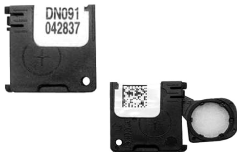
Fig. 1. Nanodot dosimeters. At the right, the rounded photoluminescent crystal is shown.
