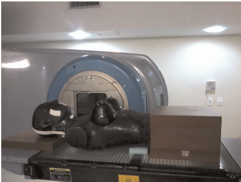
Fig. 1. Female Alderson anthropomorphic phantom used to simulate the pregnant patient. The phantom abdomen region was substituted by solid water plates.
