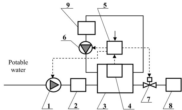
**Fig. 1.** Block diagram of a designed mineral nutrition system for PGF Vitacycle-T. 1, 6 – peristaltic pumps; 2 – enrichment column with GMRI BIONA-312™; 3 – mixing vessel; 4 – conductivity meter; 5 – regulator; 7 – electric valve; 8 – root module with FIERS BIONA-V3™; 9 – enrichment column with SAF Osmocote 14-14-14™.
