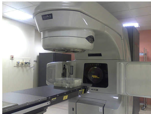
Fig. 1. Varian model Clinac 2100C linear accelerator of the Hospital Israelita Albert Einstein.
