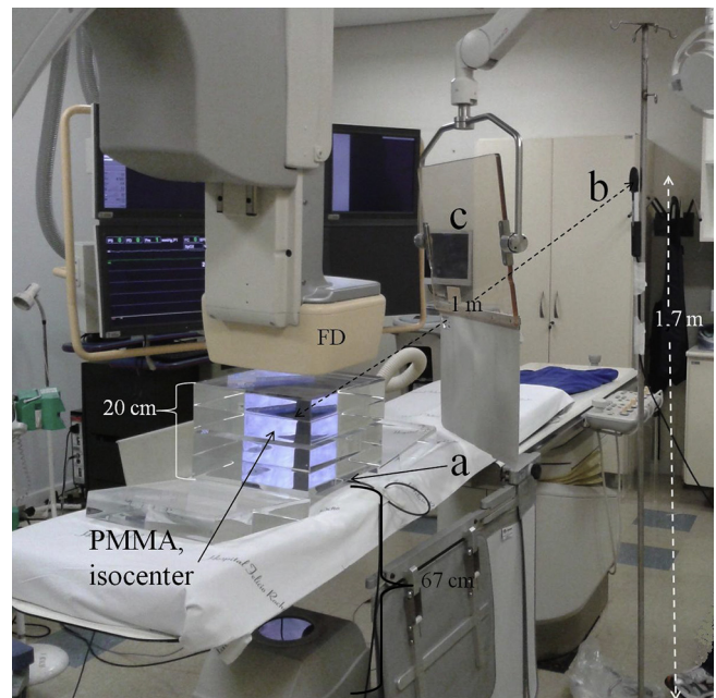
Fig. 1. Experiment arrangement, AP projection with use of a PMMA phantom of 20 cm, for measurement of phantom entrance dose (ESAK) (a) and scatter dose (b). Ceiling-suspended screen (c) and Flat panel detector (FD) (overcouch).
