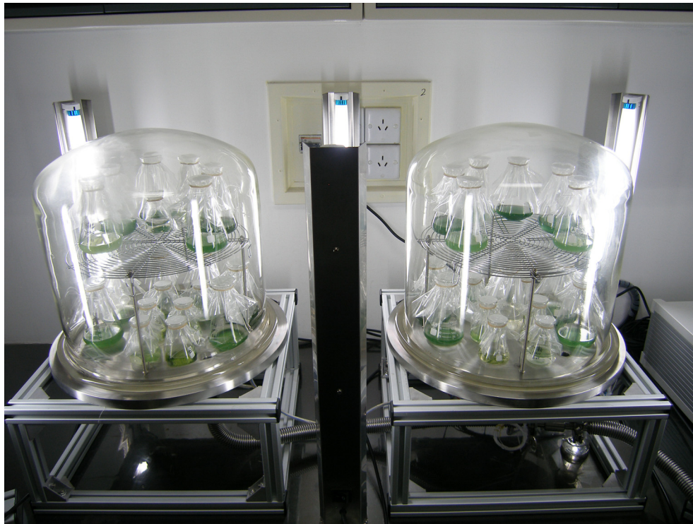
Fig. 1. Photograph of the low pressure bacteria culture facility.
