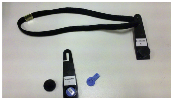
Fig. 1. Personal dosimeters to evaluate eye lens doses ( H_p(3) ).
