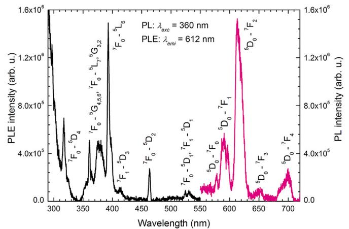
Fig. 1. PL and PLE spectra of LTB:Eu,Mn (360 nm excitation/612 nm emission).
