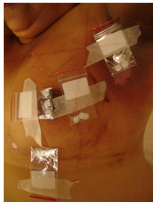
Fig. 3. LiF TLD-100H chips were placed onto a patient's skin in 4 parts. (Color version of figure is available online.)
