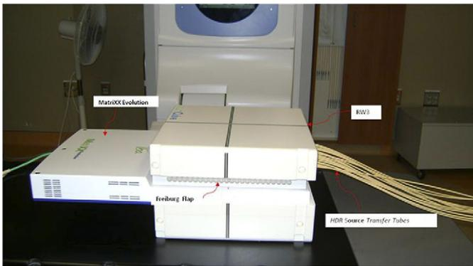
**Fig. 1.** The CBCT scan and measurement setup of IBA MatriXX Evolution. RW3 (thickness of 0, 1.0, 2.0 cm) added between the Freiburg Flap and the detector array.
