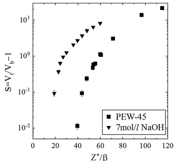
Fig. 3. A detailed response curve of CR-39 PNTD etched by PEW-45 solution at the temperature of 70 °C. The response curve obtained by 7mol/l NaOH etching at the temperature of 70 °C is also shown as a reference.
