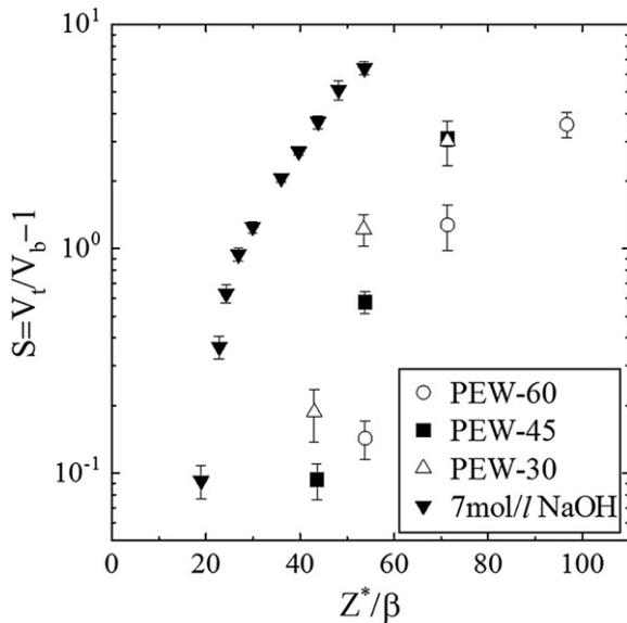
Fig. 1. The variation of track registration sensitivity for four concentrations of the PEW etchant as a function of  $Z^*/\beta$ .
