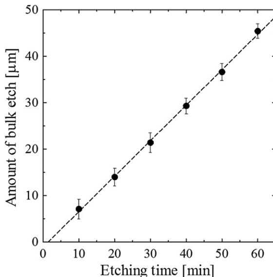
Fig. 2. The relationship between etching time and the amount of bulk etch of the CR-39 detector etched by PEW-45 solution.  $V_b$  is 0.76  $\mu\text{m}/\text{min}$  (i.e. 45.6  $\mu\text{m}/\text{h}$ ).
