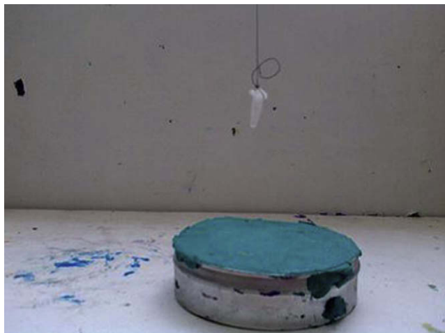
Fig. 2. Measurement of the insulation quality of plasticine on a charcoal canister using a known emanation-rate radon source.
