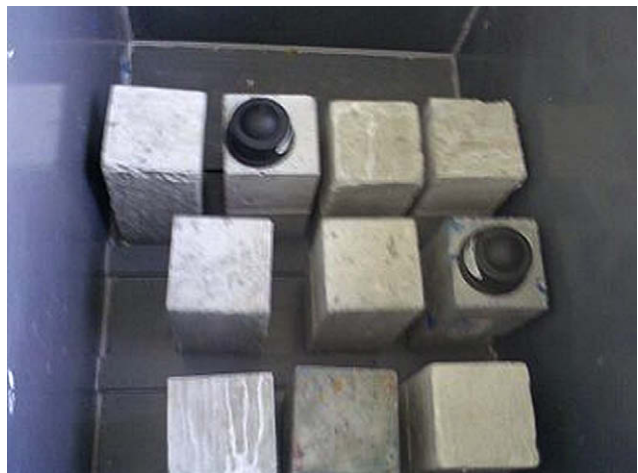
Fig. 3. Measurement of radon emanation deduced from ten open prisms using Electret detectors in a hermetically closed chamber.
