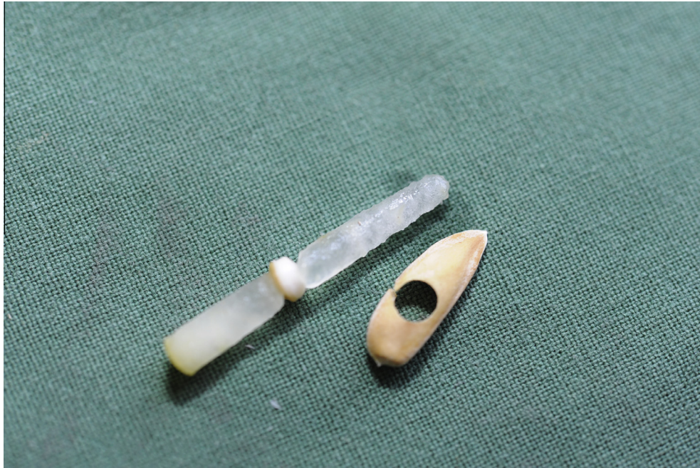
Fig. 1. Demonstration of system precision on a melon seed.
