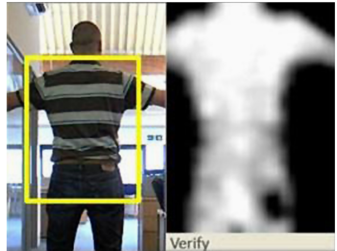
Fig. 2. CCTV and enhanced images of a passenger with a wallet in his hip pocket.
