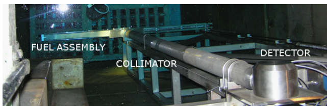
Fig. 1. Top view of the spectrometry assembly with the fuel in the fuel holder (horizontal), collimator and the detector holder located in pool “A”.
