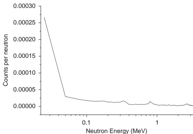
Fig. 2. Backscattered neutron flux as a function of the neutron energy. The TNT is buried 3 cm under the soil and the detector was without a shield.
