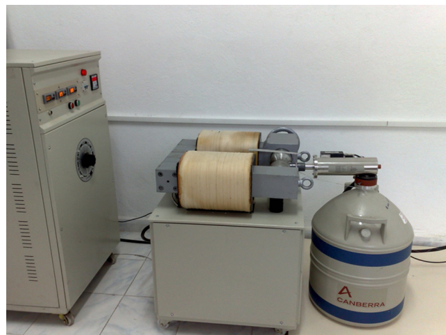
Fig. 2. Experimental setup used for measurement of La/LI , La/L\beta and La/L\gamma intensity ratio and line parameter changes.
