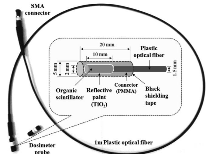
**Fig. 1.** Structure of a dosimeter probe of the SFOD.
