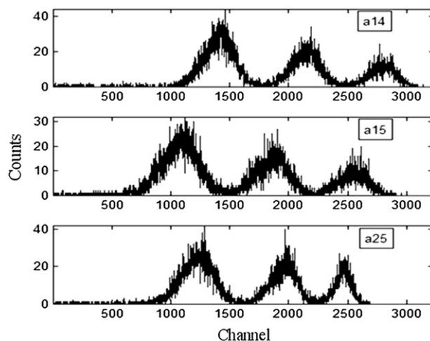
**Fig. 3.** Response of the selected SiC Schottky diodes with the same area (a14, a15 and a25) exposed in air to a mixed alpha source  ${}^{239}\text{Pu}/{}^{241}\text{Am}/{}^{244}\text{Cm}$ . The number of registered counts for each channel is represented. The measurements are referred to a counting time of 14,400 s.
