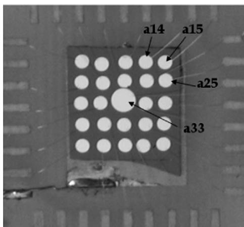
**Fig. 2.** Photograph of the  $5 \times 5$  matrix of Schottky diodes (the four diodes with the lowest reverse current density are indicated).
