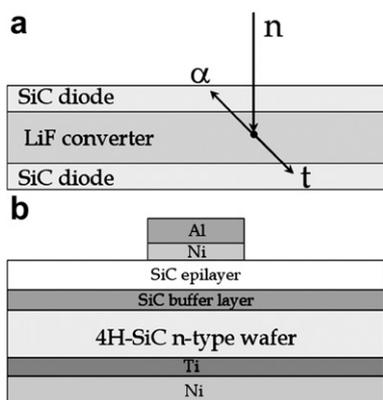
**Fig. 1.** a) Schematic representation of the sandwich neutron spectrometer (dimensions are not to scale). The  ${}^6\text{LiF}$  reaction is considered (a thermal neutron incident on the spectrometer is represented in the scheme). b) Scheme of each Schottky diode which was realized on the 4H-SiC wafer (dimensions are not to scale).
