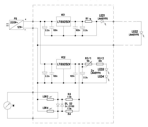
Fig. 1. Circuit diagram of the GaAs-LED based neutron monitor.
