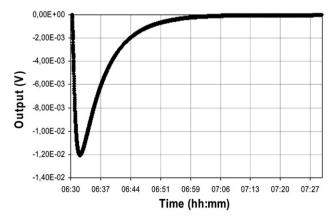
Fig. 4. Warm-up behaviour of the GaAs-LED based neutron fluence monitor.
