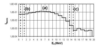
**Fig. 3.** Monte Carlo calculated neutron spectrum from [d(14)+Be] reaction (a), in addition line spectra of 1 MeV neutrons (b) and 14 MeV D+T fusion neutrons (c).
