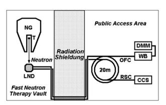
Fig. 2. Schematic setup of the real-time neutron fluence monitoring experiment.
