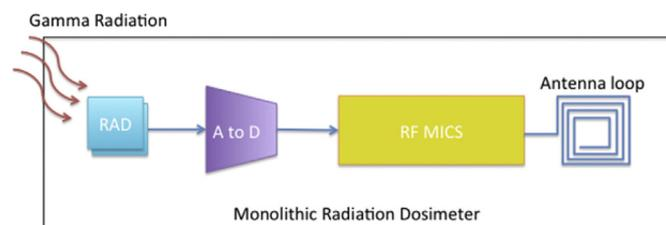
Fig. 1. Block diagram of the monolithic dosimeter.
