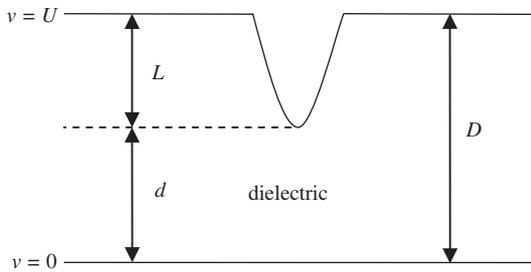
Fig. 1. The track geometry and boundary conditions.
