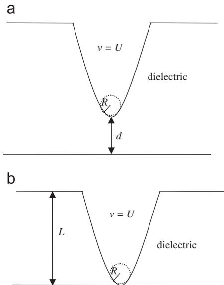
Fig. 2. Track geometry used in (a) Mason's equation, (b) Smythe's equation.
