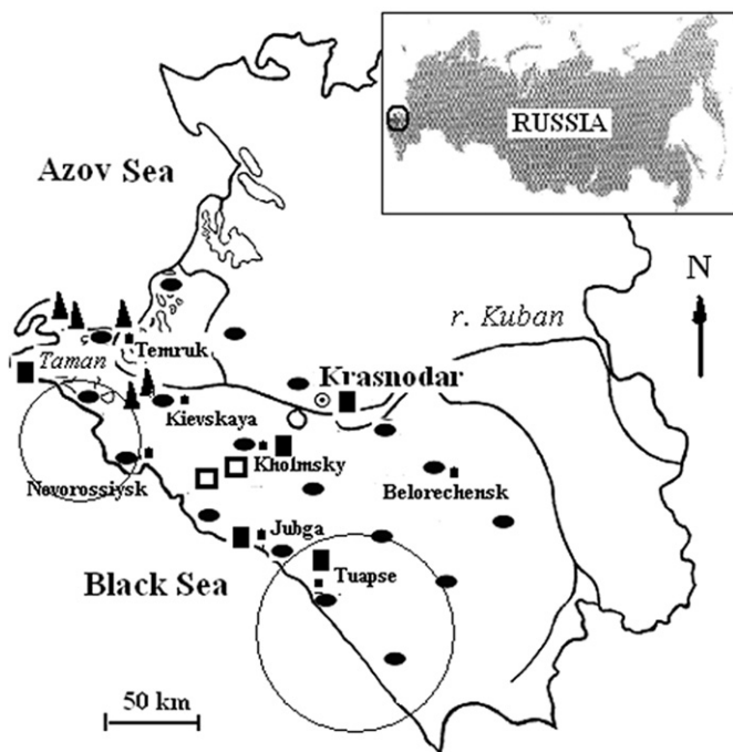
Fig. 1. Map of the Rn observation station in the Western Caucasus. Black squares show points in the faults; white squares show points in mineral deposits; triangles designate mud volcanoes; points of the Rn-network are shown by black ellipses. The large circles show seismically active zones. The region of study is shown by a circle on the map of Russia.
