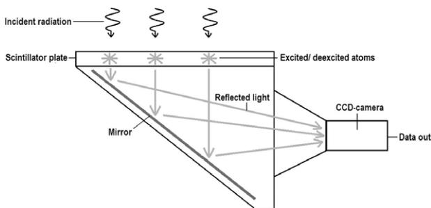
Fig. 2. Schematic illustration of the performance of the BIS-2G detector system.
