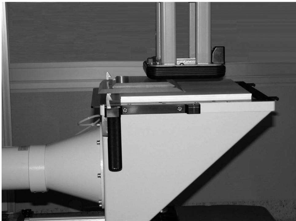
Fig. 3. A photo of the measurement setup showing a 20-mm-thick bolus edge with a  $30^\circ$  angle placed on 2-cm buildup on the BIS-2G.
