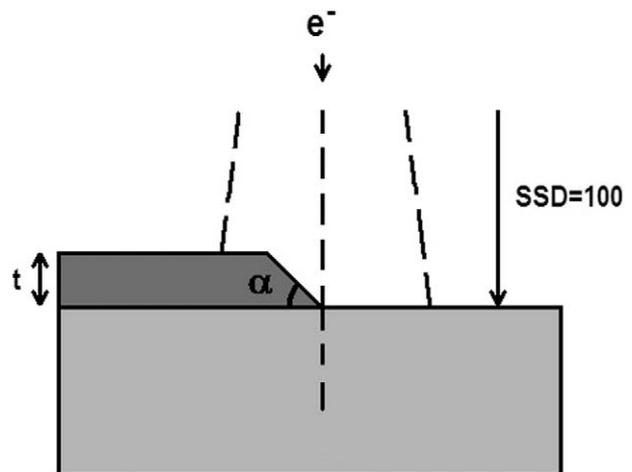
Fig. 1. Schematic illustration of the measurement geometry illustrating the positioning of the bolus in the irradiated field, with the thickness of the bolus ( $t$ ), the angle of the bolus edge ( $\alpha$ ), and the source-to-surface distance (SSD).
