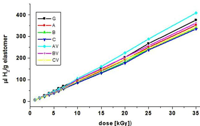
**Fig. 1.** Volume of hydrogen formed in the result of irradiation of granulate and sheets of elastomers.
