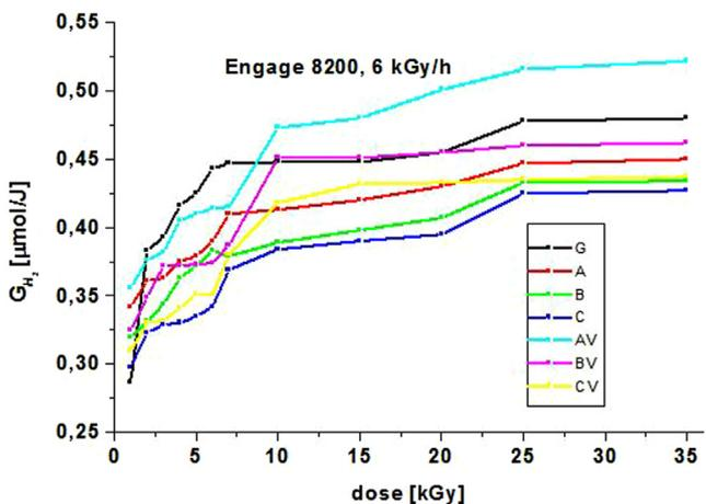
**Fig. 2.** The yield of hydrogen and the yield of absorbed oxygen vs absorbed dose.
