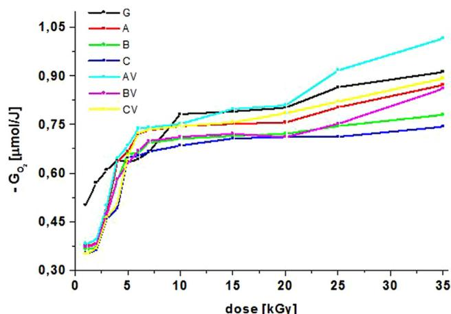
**Fig. 3.** The yield of hydrogen and the yield of absorbed oxygen vs absorbed dose.
