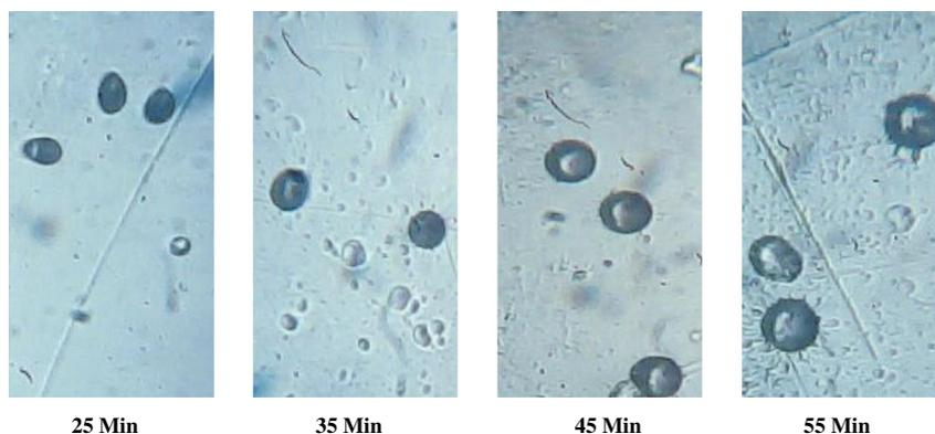
Fig. 1. Typical optical images of fission tracks in the DAM–ADC detector with etching condition (8 ml of 10 N NaOH + 1 ml CH<sub>3</sub>OH) at 60 °C.
