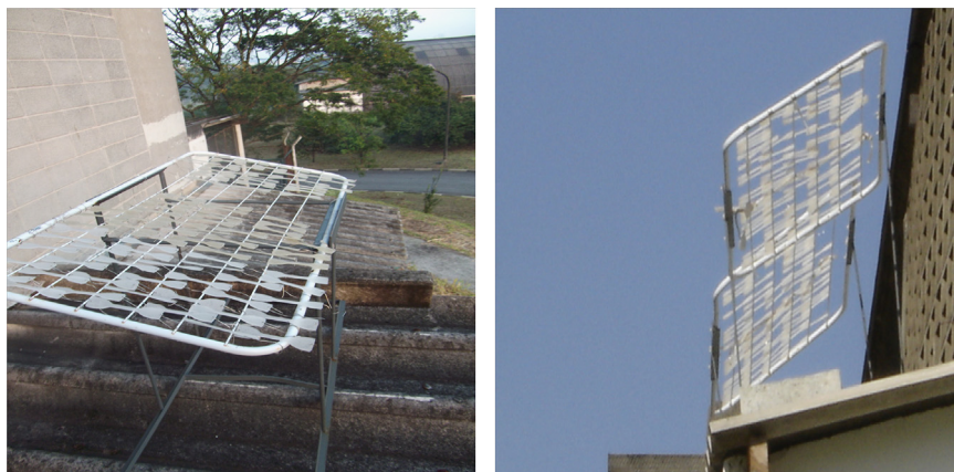
Fig. 1. Device with dumbbell samples for environmental ageing exposed outside at the polymer processing laboratory IPEN/CQMA.
