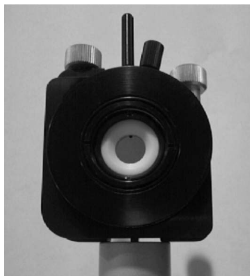
Fig. 3. Holder-mounted ZnTe [110] crystal as high resistivity EO crystal.
