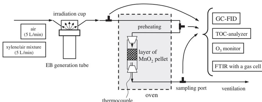
Fig. 1. Apparatus for electron beam irradiation of air and xylene/air mixture, their catalytic process using  $MnO_2$ , and analysis of these gases before and after the catalytic process.
