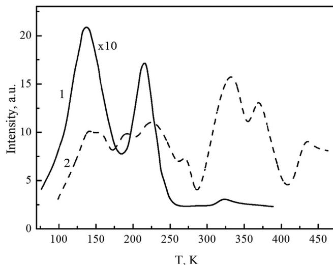
Fig. 1. TSL of  $LiKSO_4$  crystal irradiated by X-rays(1) and 6–6.2eV photons (2) at the temperature of liquid nitrogen.
