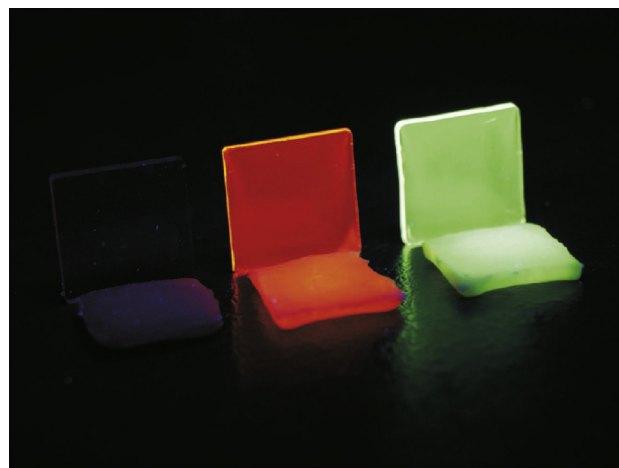
Fig. 1. REdoped borate glasses (upright) and glass ceramics (lying): undoped (left), \text{Eu}^{3+} doped (middle), and \text{Tb}^{3+} doped (right) under ultraviolet irradiation. The undoped reference glass does not show any luminescence.
