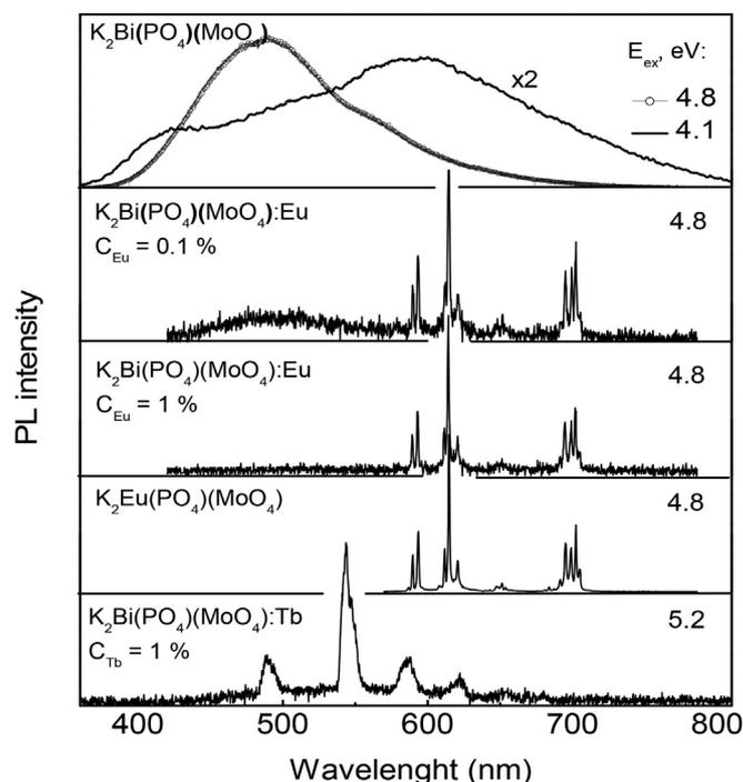
Fig. 1. The PL emission spectra of undoped, Eu- and Tb-doped K<sub>2</sub>Bi(PO<sub>4</sub>)(MoO<sub>4</sub>) crystals, T = 8 K, excitation photon energies E<sub>ex</sub> are indicated in the figure.
