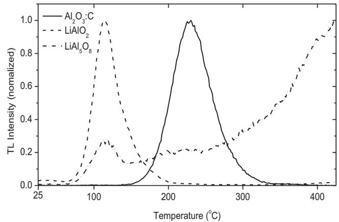
**Fig. 3.** TL glow curves of  $\text{Al}_2\text{O}_3\text{:C}$ ,  $\text{LiAlO}_2$  and  $\text{LiAl}_5\text{O}_8$  irradiated to 900 mGy beta rays from  $^{90}\text{Sr}$ – $^{90}\text{Y}$  and recorded on Risoe reader (heating rate 5 °C/s).
