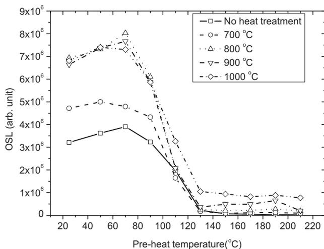
**Fig. 2.** Effect of heat treatment for 30 min before irradiation and pre-heat before readout (in the OSL reader) on OSL sensitivity of  $\text{LiAlO}_2$ . The OSL sensitivity is represented by an integration of CW-OSL signal for the first 10 s during readout for 40 s.
