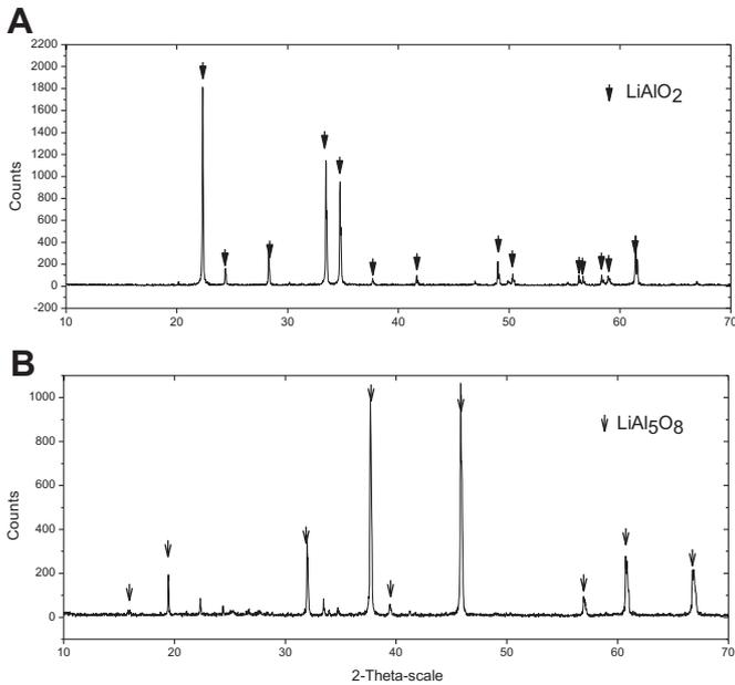
**Fig. 1.** Results of X-ray diffraction analysis of Ir crucible melt (dominated by  $\text{LiAlO}_2$  formation, Fig. 1A) and graphite crucible melt (dominated by  $\text{LiAl}_5\text{O}_8$ , Fig. 1B) with all other parameters remaining the same.
