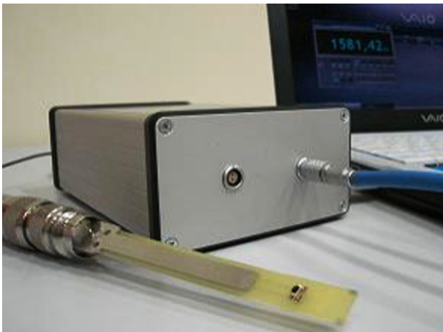
Fig. 1. The dosimetry system: phototransistor on a printed circuit board, the Flip-flop electrometer, a computer and the DoseX ® software.
