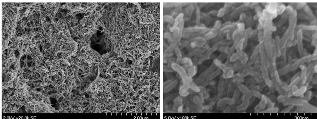
**Fig. 1.** SEM of dropcast ink containing single walled carbon nanotube, tetrabutylammonium bromide (TBAB) modified Nafion<sup>TM</sup>, 1-pyrenebutanoic acid, succinimidyl ester (PBSE), and bilirubin oxidase on glassy carbon. Scale bar 2  $\mu\text{m}$  (left) and 300 nm (right).
