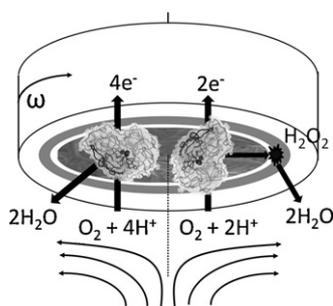
**Scheme 1.** 4 and 2 electron transfer on the carbon nanotube coated rotating ring-disk electrode.
