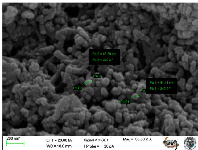
Fig. 1. SEM image of the P(2ClANI)/PANI copolymer nanoparticles.
