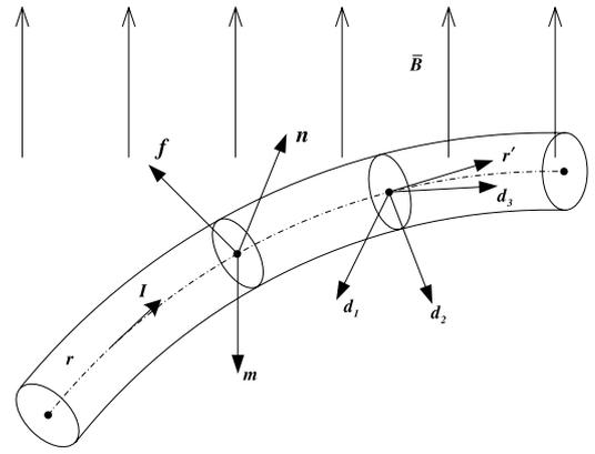
Fig. 1. Schematic diagram of a Cosserat rod.
